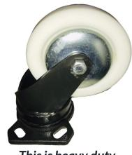
This is heavy duty forged steel caster. Steel balls are accommodated between two ball races. The top forged swl base plate is interlocked by these steel balls with the inner ring part of the cup which serves both as thrust and taper bearing.
